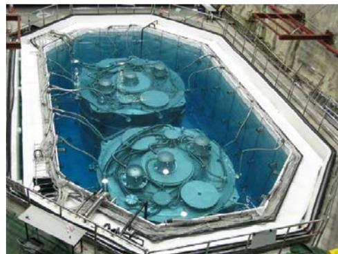
Figure 1: a) Top view of the interior of the Daya Bay Antineutrino Detector. b) View of one of the three Daya Bay experimental hall after the two ADs were installed in the water pool.
